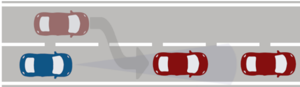
Figure 33: Schematic representation of test scenario UC 2-C (TJC cut-in).
