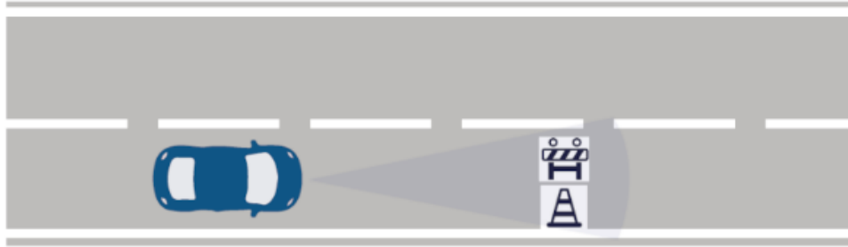
Figure 35: Schematic representation of test scenario UC 2-E (TJC blocked lane by stationary object).
