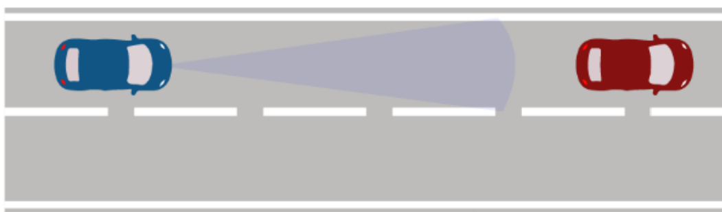
Figure 32: Schematic representation of test scenario UC 2-B (TJC speed limit adaptation to vehicle ahead).
