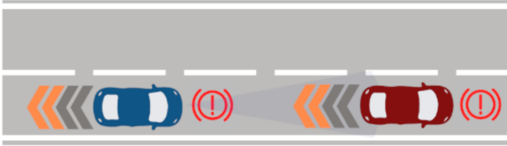
Figure 39: Schematic representation of test scenario UC 2-I (TJC emergency deceleration).
