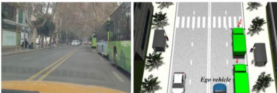
Figure 27: Scene illustration of sub-UC 1.3-A “Darting-out pedestrian” scenario (straight road segment).
