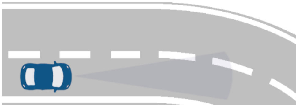
Figure 42: Schematic representation of test scenario UC 2-L (Lane keeping while entering a curve).
