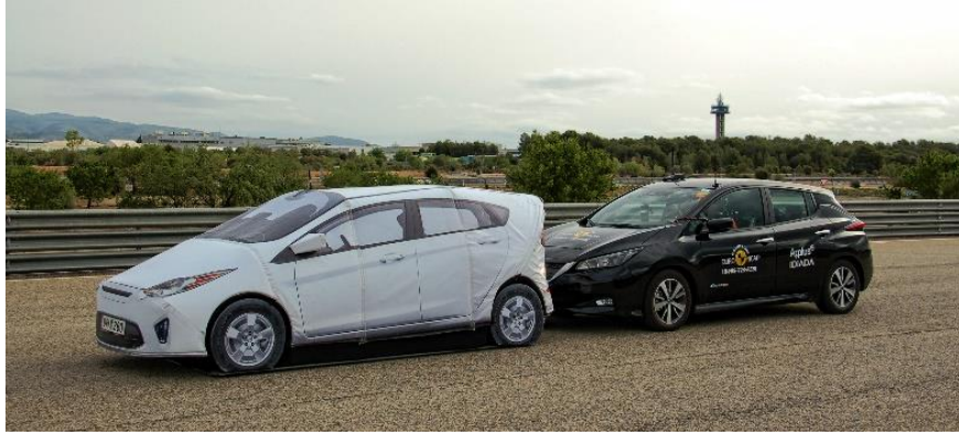
Figure 29: Euro NCAP AEB test on proving ground (potential collision of real drivers with target, source: Applus IDIADA)
