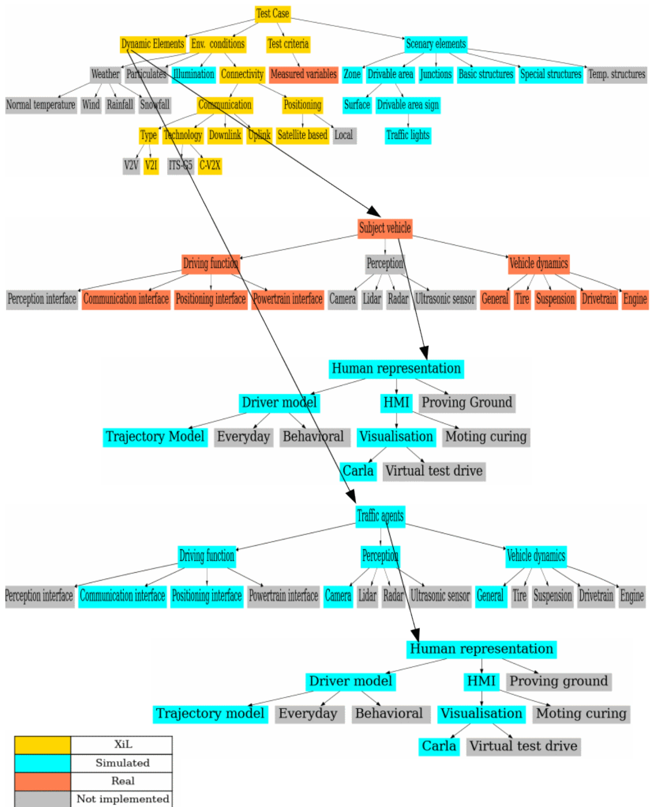
Figure 44: Test instance structure of sub-UC 1.3-B “urban junction”
