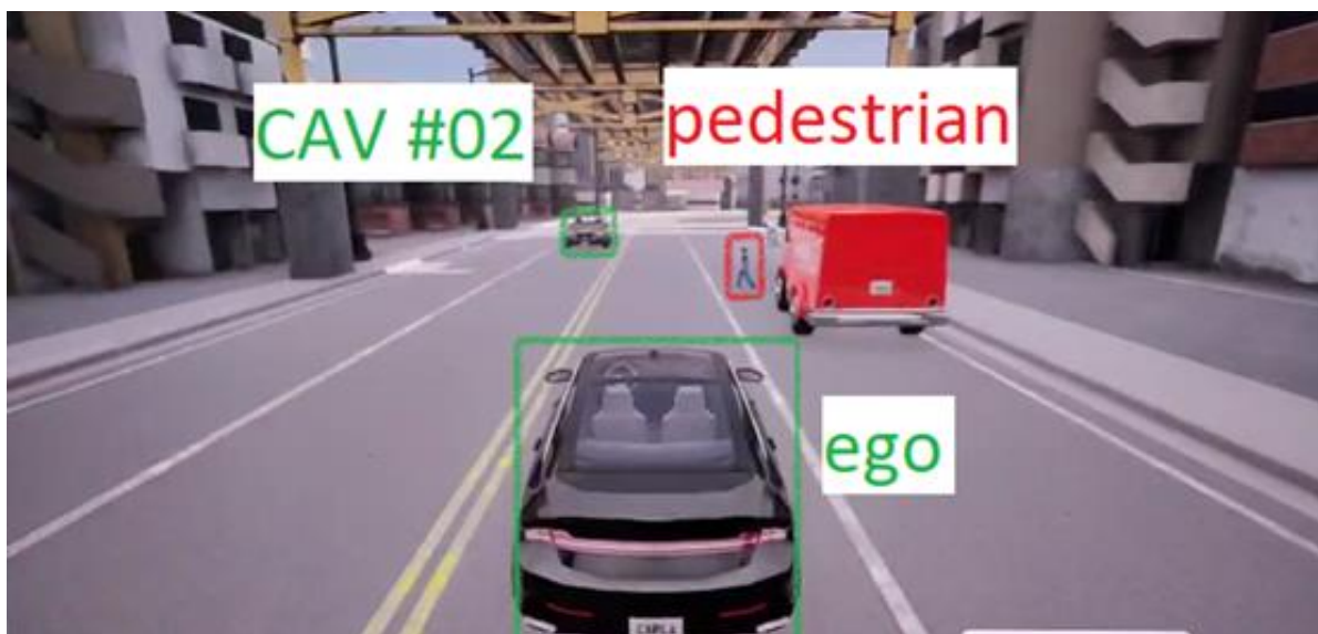
Figure 41: Schematic representation of sub-UC 1.3-A "darting-out pedestrian" test scenario
