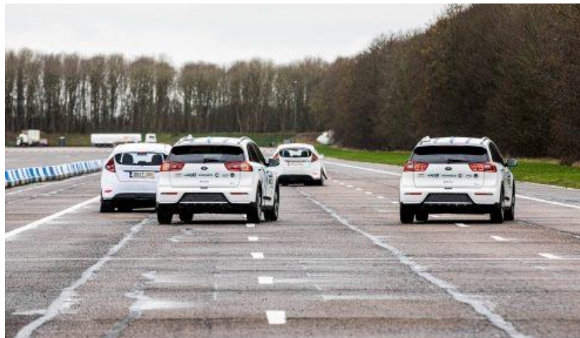
Figure 30: Proving ground testing with safety drivers as backup solution in case of ADS faults to prevent collisions (source: MuCCA project)
