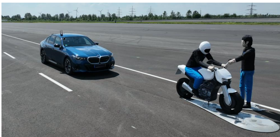
Figure 30: Proving ground testing setup with VUT, Motorcycle and Pedestrian Dummy in a blocked lane scenario
