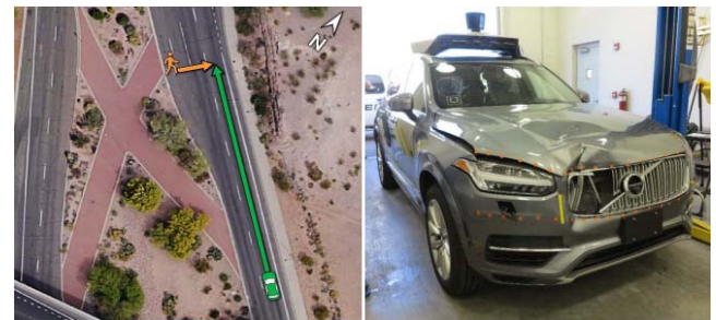
Figure 3: Aerial view of crash location showing the path of VRU (orange) and car (green). On the picture on the right, the deformation on the front face of the car due to the crash.
