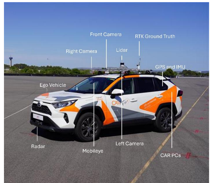
Figure 3 Exterior image of the CAVKit vehicle with all the sensors available for the perception and localization systems
