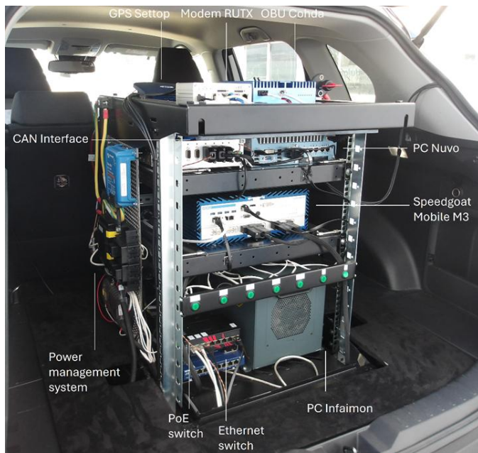
Figure 2 CAVKit rack with all the devices placed in the trunk
