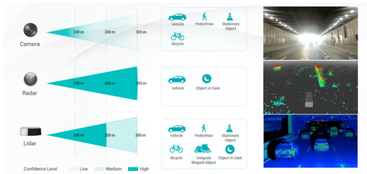
Figure 22: Comparison of LiDAR specifications with respect to camera and radar [21]
