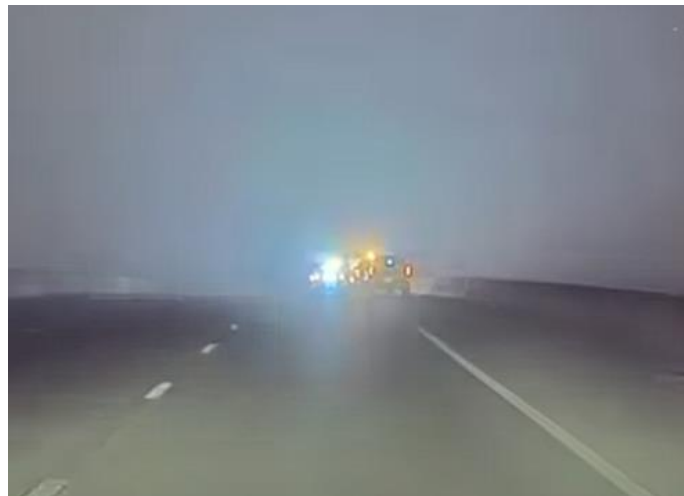
Figure 33: Dash camera footage prior to a Tesla autopilot crash. The blooming effect due to headlights of the emergency vehicles parked in front may have been a contributing factor [32] .
