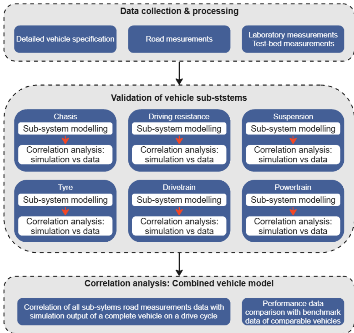
Figure 13: Schematic overview of vehicle sub-systems validation flow
