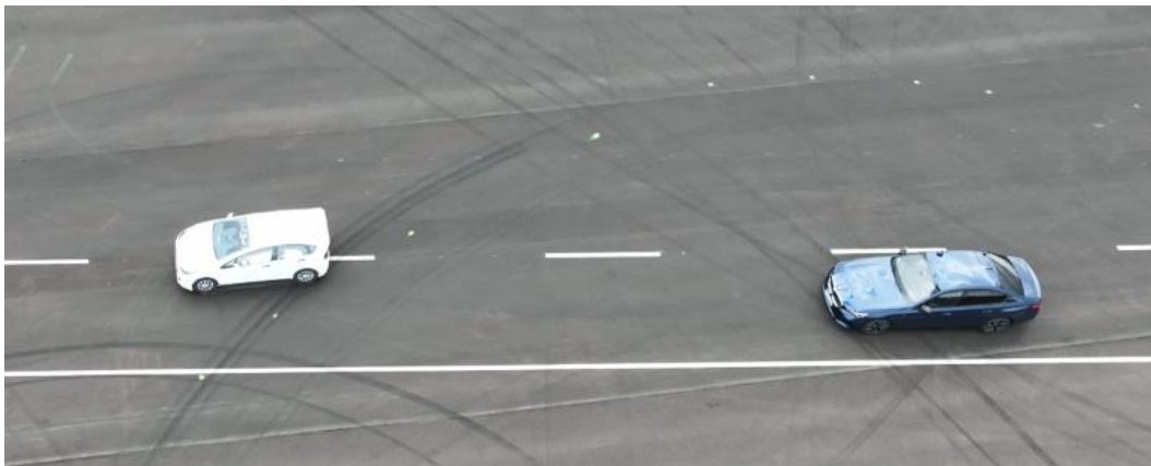
Figure 7: Set-up for proving ground testing with crashable soft car target and ego vehicle
