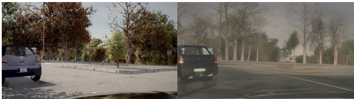
Figure 25: Left: Camera sample generated by the CARLA simulator. Right: Rendered image by the photorealistic AI.
