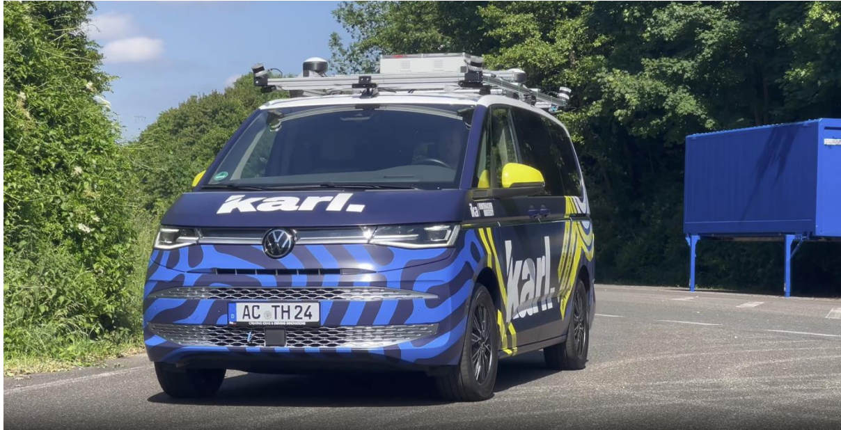
Figure 48: ika's automated vehicle test platform karl.
