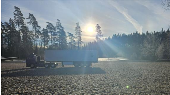
Figure 219: A test scenario with sun elevation of 9° in a hardware-in-the-loop scale truck environment.
