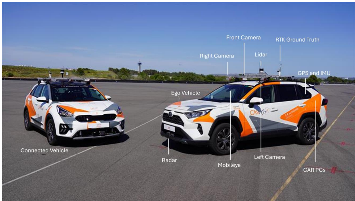
Figure 163: Use Case 3.2: Cooperative Vehicle and Ego Vehicle used.
