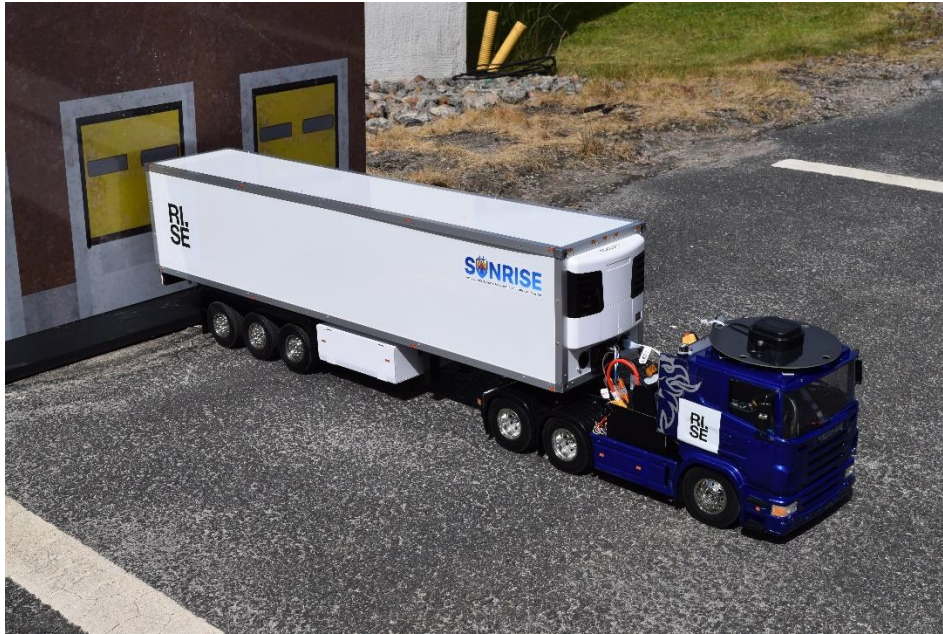
Figure 206: Photo of the 1:14 model truck with a semitrailer. On the roof of the truck is the GNSS antenna.
